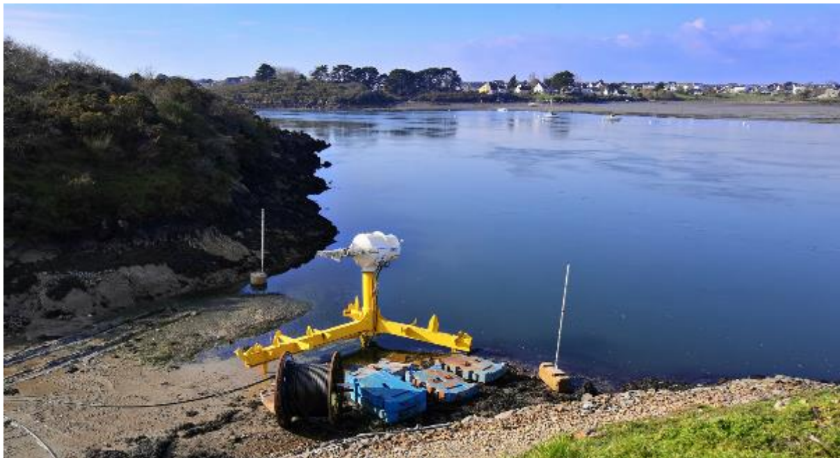
Photo 3 – NOVA's tidal turbine RE50 visible during the site visit, before the deployment in the Etel estuary
