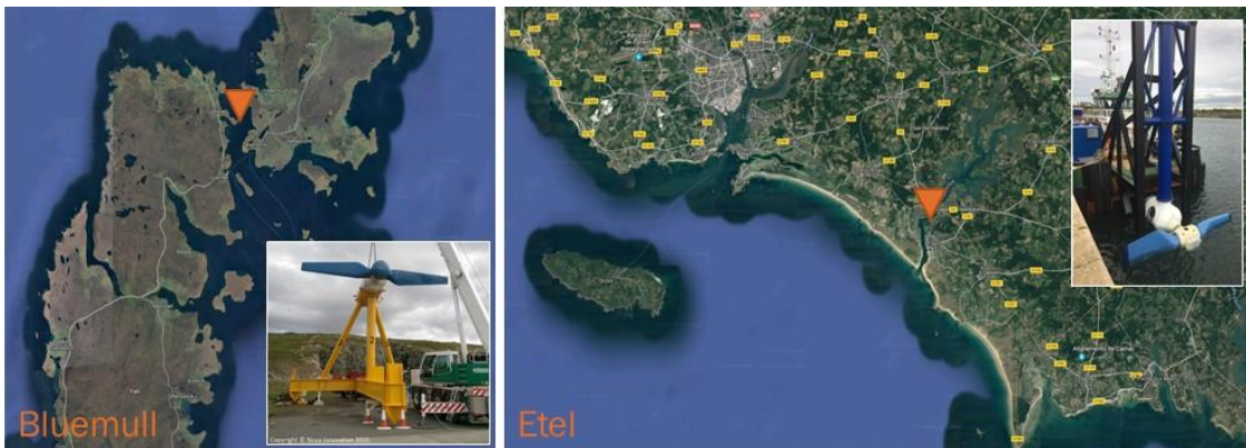
Figure 2. Precise localization of the Bluemull and the Etel test sites (maps) where the type of device that is currently deployed (M100, 3 turbines, Bluemull) and that is planned to be deployed (Nova RE50, 1 turbine, Etel).
